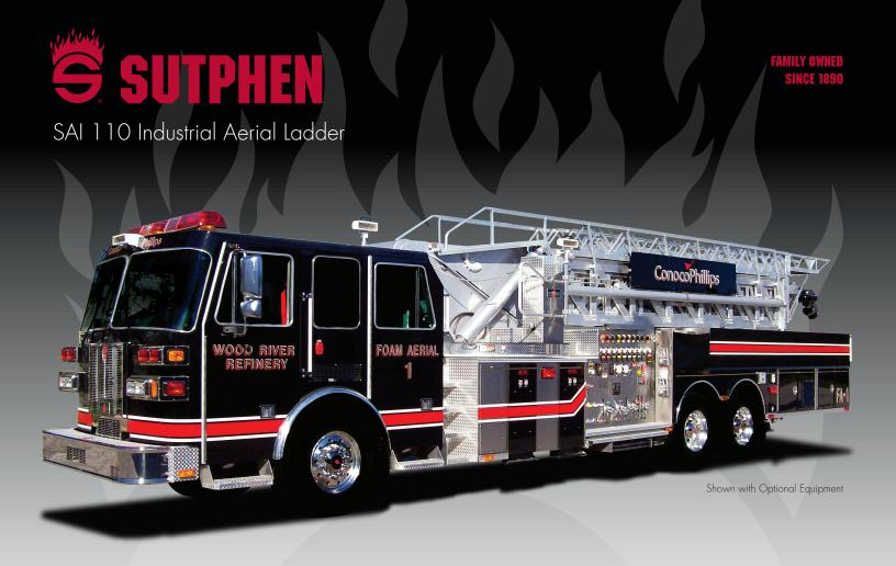
Sutphen Petrochemical and Industrial Aerials are the industry's most reliable, and most demanded apparatus on the market. Sutphen is the leader in highest flow, highest elevation, and workable foam streams for industrial firefighting. The Sutphen aerial can flow up to 4000 gpm at 100' of elevation from a pressurized water source, a feature unmatched by any other manufacturer.
