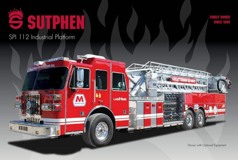
Sutphen Petrochemical and Industrial Aerials are the industry's most reliable, and most demanded apparatus on the market. Sutphen is the leader in highest flow, highest elevation, and workable foam streams for industrial firefighting. The Sutphen aerial can flow up to 4000 gpm at 100' of elevation from a pressurized water source, a feature unmatched by any other manufacturer.
